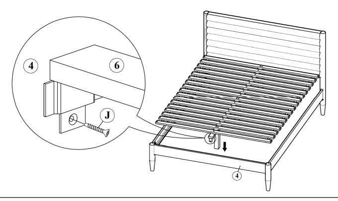
STEP 6: Attach Assembled Bed Slats to Assembled Bed Frame with (F) Using a Allen Key M4 (A) as shown.
