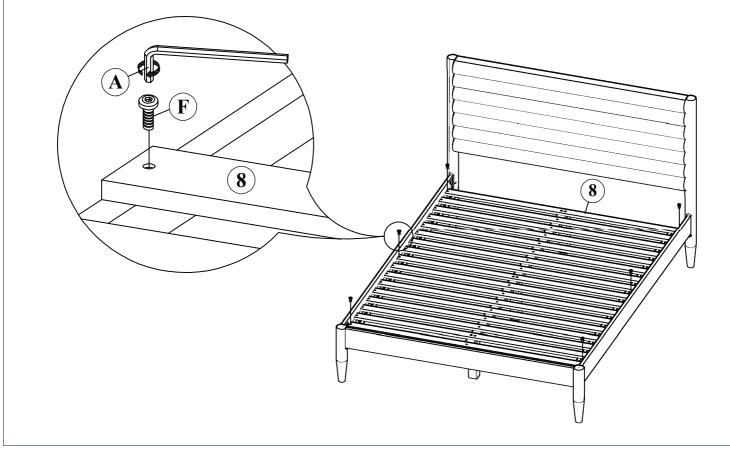
STEP 7: Attach Assembled Bed Slats to Assembled Bed Frame with (K) using a Screwdriver as shown.
