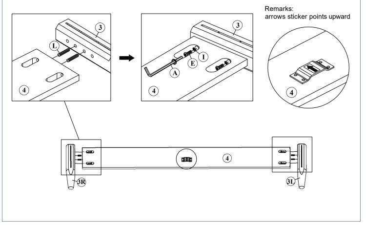
STEP 3: Attach (5) to (2) and (3) Assembled Headboard and Footboard as shown.
